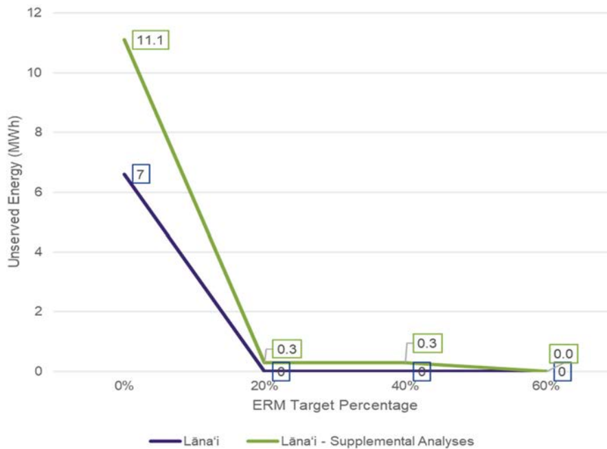
Figure C- 14: Lānaʻi Unserved Energy by ERM Percentage for PLEXOS Stochastic Outage Production Simulation
