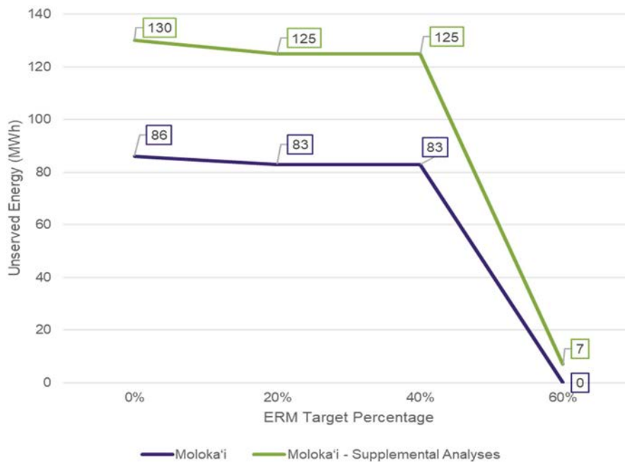
Figure C– 17: Moloka‘i Unserved Energy by ERM Percentage for PLEXOS Stochastic Outage Production Simulation
