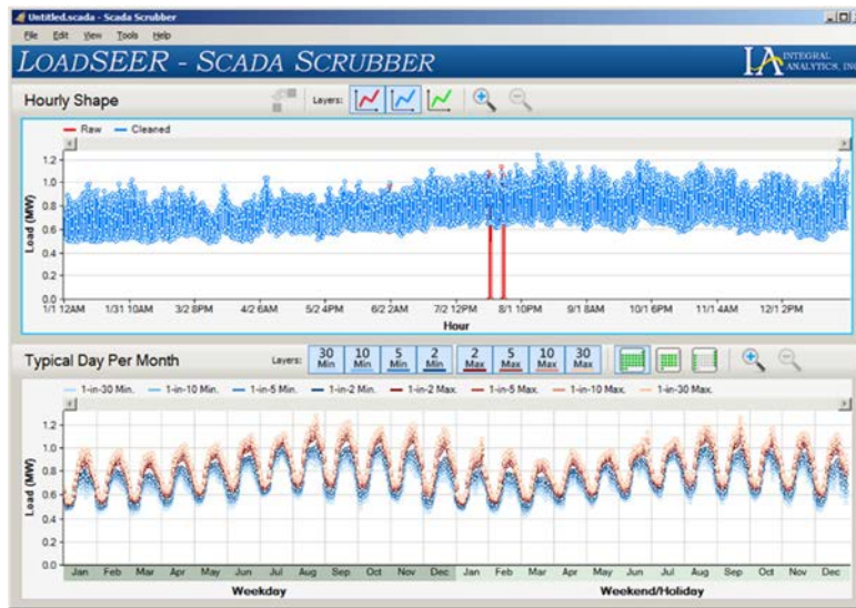
Figure I- 3: LoadSEER SCADA Scrubber Screenshot
