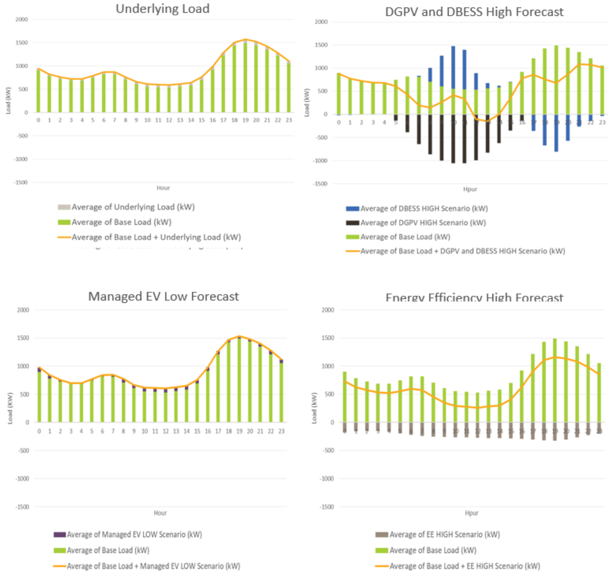
Figure 27: Scenario 3 Average Daily Hourly Load Profiles by Layer (Underlying Load, DGPV and BESS, EV, and EE) with Stacked Load for Sample Circuit
