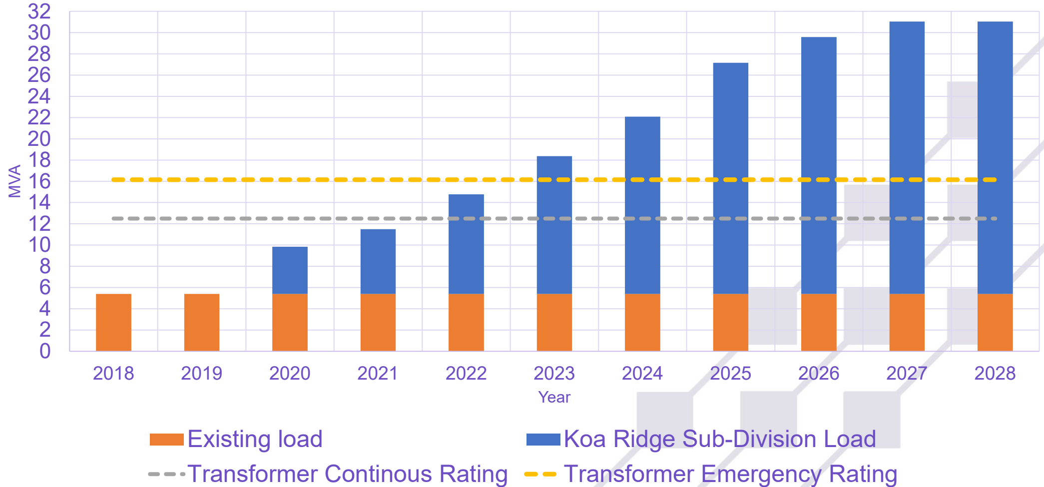
Waipio Ckts Load Growth and Transformer Ratings
