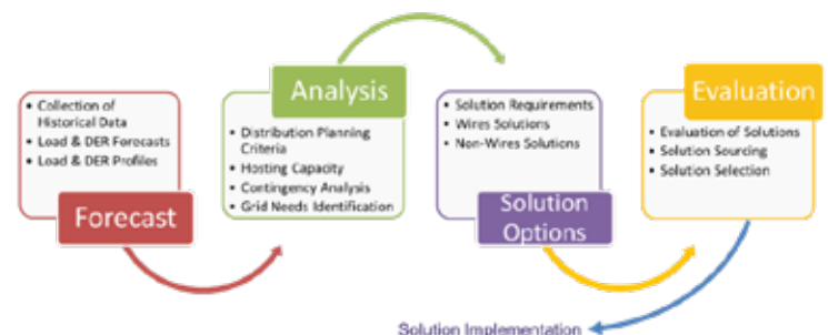
Figure 1: Stages of the Distribution Planning Process
