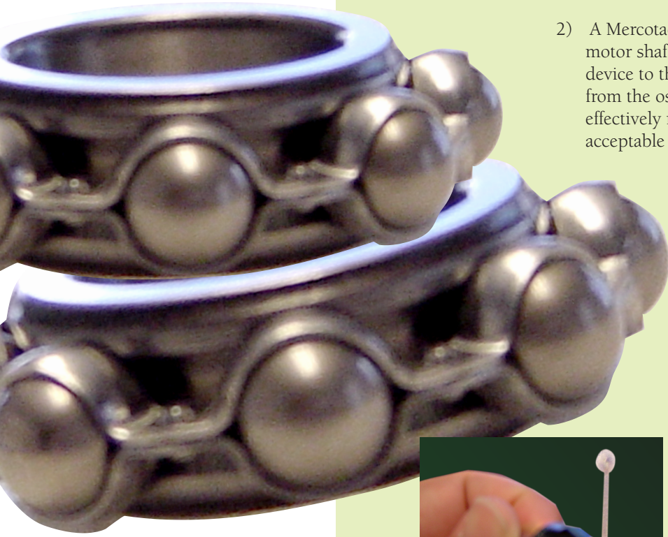
Fig. 2: Bearings beginning to show signs of surface "frosting"
